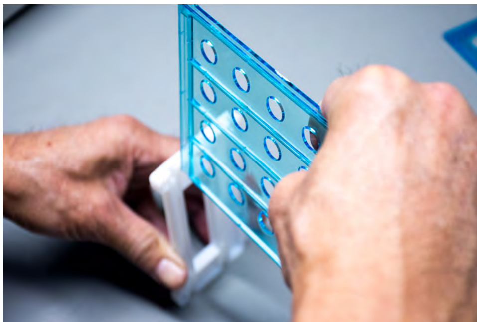
Now take the bottom layer and with the groove opening on the side of the layer facing towards you, insert it into the bottom groove of the side piece (left-hand side shown)
